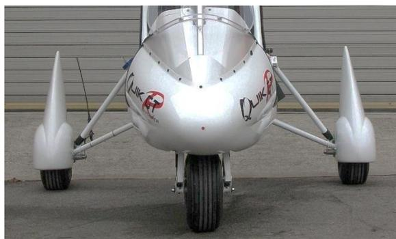
New for the Quik range of trikes a set of new wheels with a larger footprint than standard allowing for a better rough field performance. Large Tundra tyres 6 inches wide with revised pod and wheel spats to suit.
