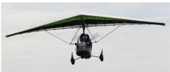
A 13sqm topless wing offering good all round speeds, standard on the PulsR and available for the original Quik range of trikes (subject to specification). This wing offers a standard trim range of 55mph to 95mph, and fitted with STARS gives unrivalled roll controls at all speeds, whilst maintaining full stability at all loads. The wing has been tested up to a maximum take-off weight of 472.5kg so can take full advantage of the increased payload offered when a BRS parachute is fitted.
